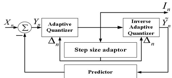
Figure 2. Conventional structure of adaptive differential encoder with backward adaptive quantizer
