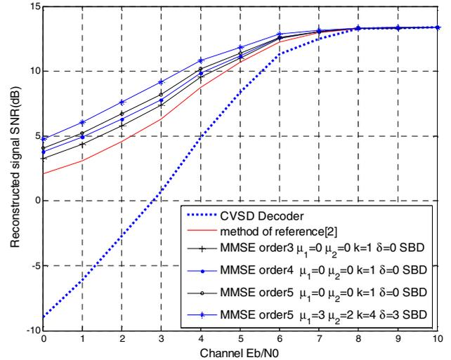
**Figure 4.** Performance of CVSD Decoder, method of [2] and proposed MMSE Decoder for order 3, 4 and 5
