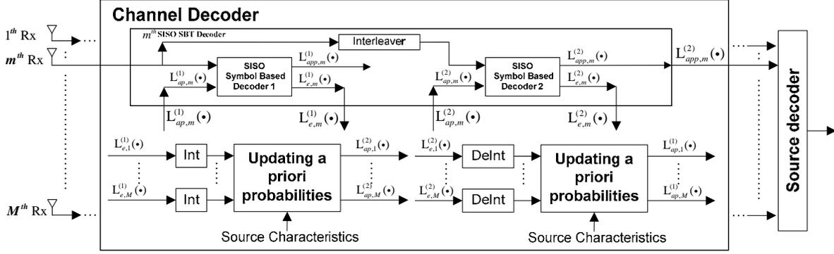
Figure 2. Structure of the receiver of MD with symbol based turbo codes.
