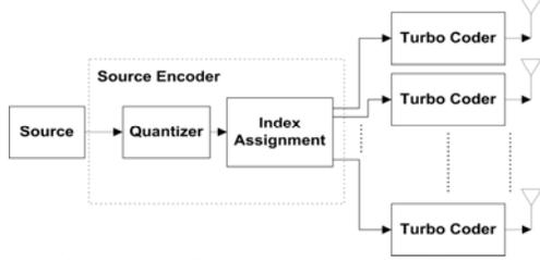
**Figure 1. Structure of the transmitter of MD with symbol based turbo codes.**
