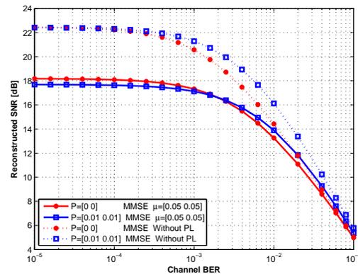
Figure 5. Performance of a MD system designed at a specific value of the equivalent channels BER, and used over channels with different BER.
