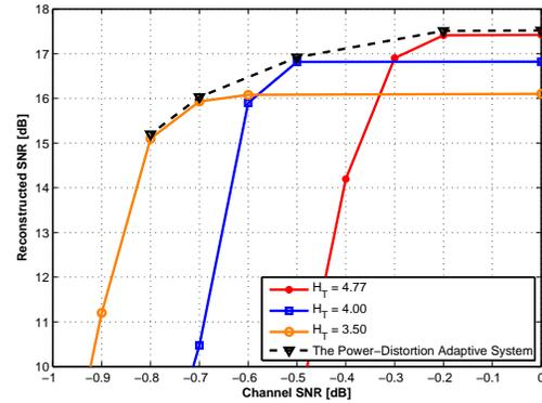
Figure 3. Performance of the JSSC system using MD with SBT codes. Three descriptions are used.
